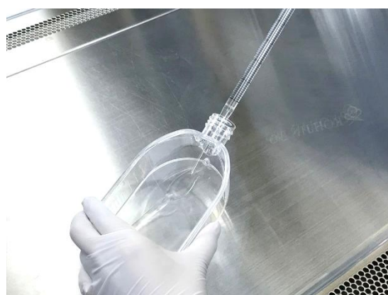
Coat a flask with the coating agent (Photo 2)
